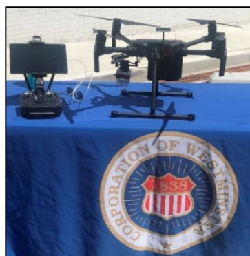
Left to Right: 1. Land Surface Temperature of Downtown Westminster; 2. Towson University quadcopter drone outfitted with a 6-band multispectral sensor; and 3. Drone photo of Downtown Westminster
